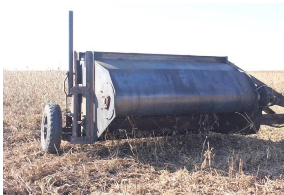
Fig. 3. Laboratory installation for stripping standing soybeans
