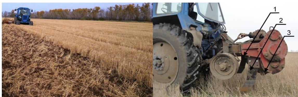
Fig. 1. Field tests of the tillage unit with a rotary plow: 1, 2 – subsoilers; 3 – rotor
